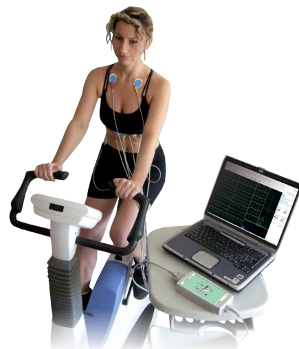
Quark C12x and T12x can also be used as standalone Stress Test ECG Measuring Stations
