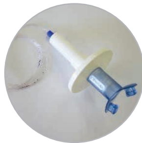
Pressure Transducer with AB filter for MIP/MEP testing
