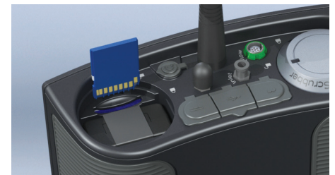
Accessing the SD-card slot is useful to simplify data sharing without connecting to the PC
